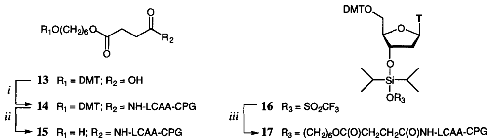
Figure 3. Improved synthesis of SLCPG 17 (40 \mu\text{mol.g}^{-1} ) via DCC/DhbtOH mediated coupling of 13 to LCAA-CPG (68 \mu\text{mol.g}^{-1} ). Reagents and conditions: i , acetic anhydride, DMAP, 2,6-lutidine; ii , ref. 5j; iii , 15 , ref. 14.
